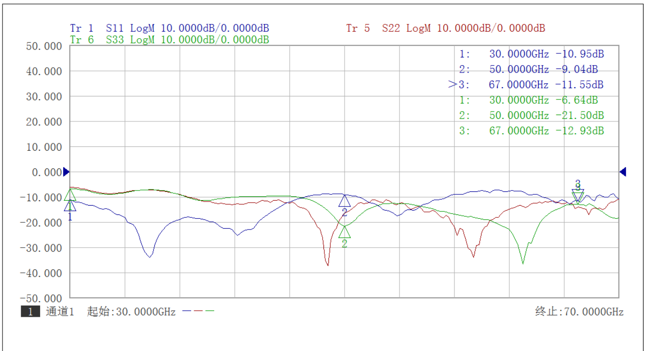
Return Loss vs Frequency State4(Both RF2/RF3 OFF)
